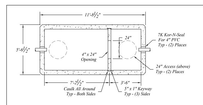
Septic Tank Sections To Be Manufactured per AASHTO 17th Ed. and ASTM Specifications w/HS-25 Loading and 0.0' to 3.0' of Earth Cover.
