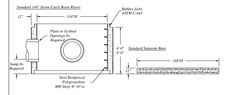
144" Manhole Pipe, Reducers, Covers and Bases Are Manufactured To ASTM C-478 Specifications.
