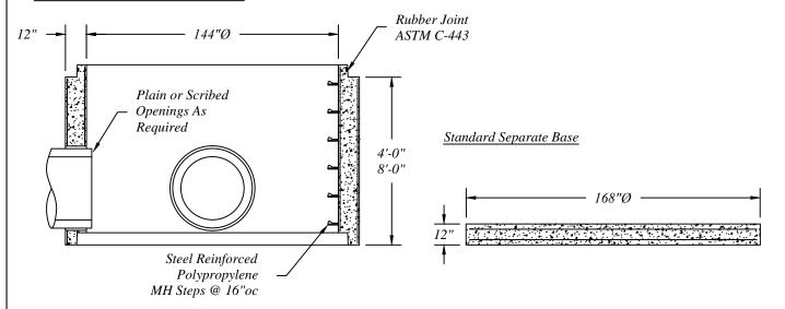
144" Manhole Pipe, Reducers, Covers and Bases Are Manufactured To ASTM C-478 Separat Specifications.
