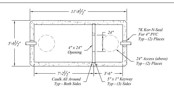
Septic Tank Sections To Be Manufactured per AASHTO 17th Ed. and ASTM Specifications w/HS-25 Loading and 0.0' to 3.0' of Earth Cover.
