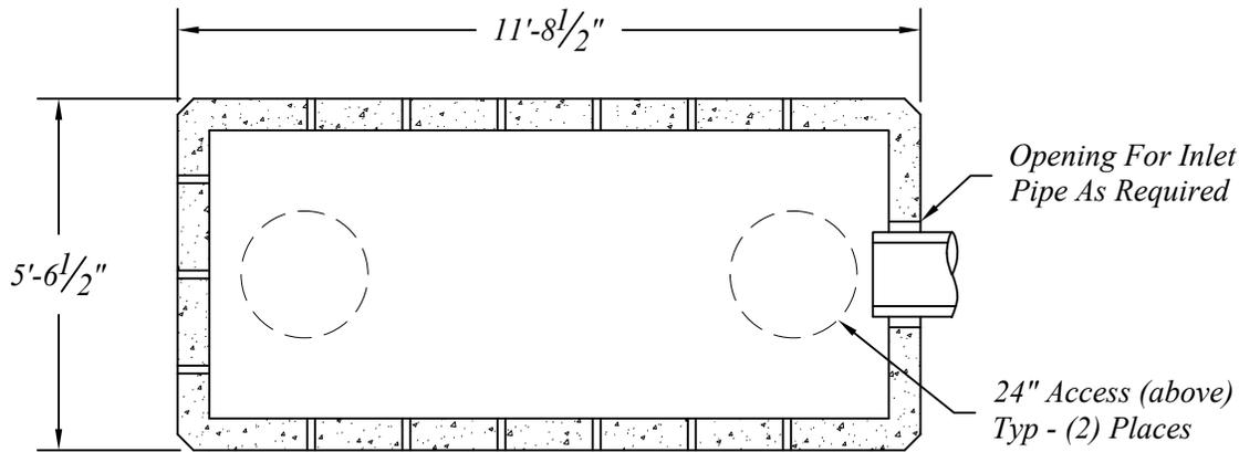
Dry Well Sections To Be Manufactured per AASHTO 17th Ed. and ASTM Specifications w/HS-25 Loading and 0.0' to 3.0' of Earth Cover.
