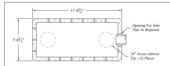
Dry Well Sections To Be Manufactured per AASHTO 17th Ed. and ASTM Specifications w/HS-25 Loading and 0.0' to 3.0' of Earth Cover.
