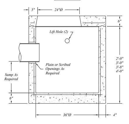
Catch Basin Sections Manufactured To ASTM C-478 Specifications.
