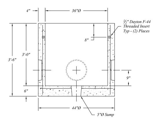
Precast Handhole To Be Manufactured To ASTM C-478 Specifications w/HS-20 Loading.
