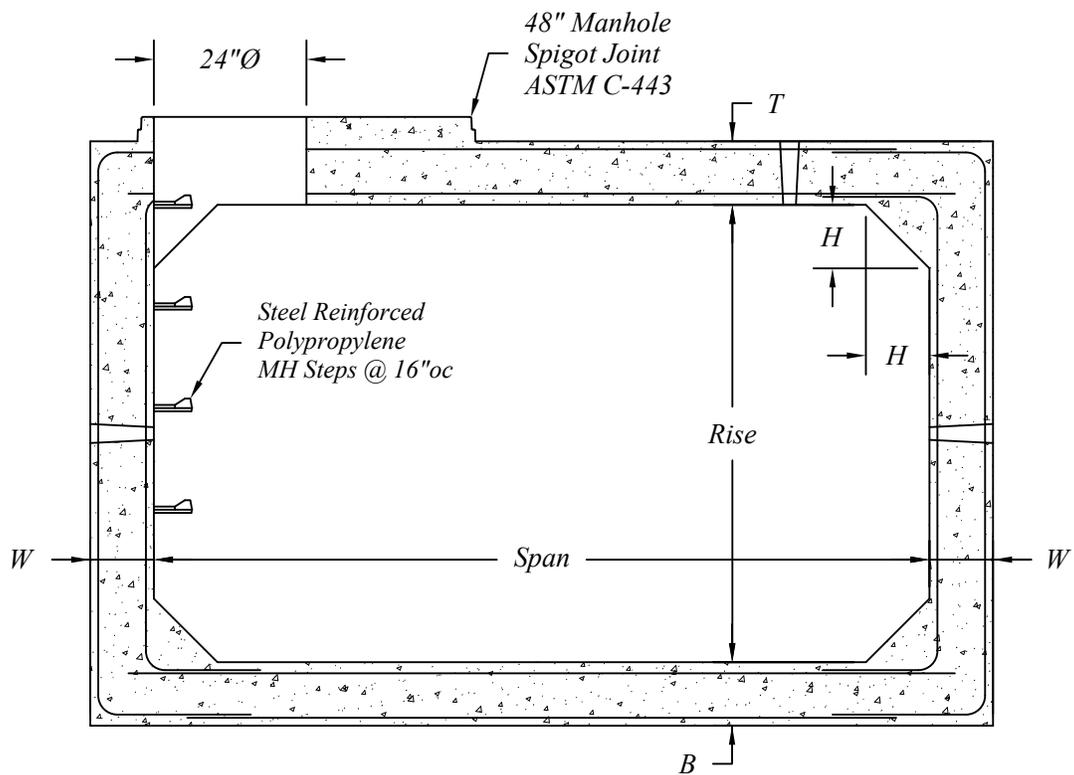
Typical Prefabricated Box Culvert Manhole Tee Detail
