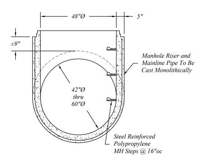
Pipe Manufactured To ASTM C-76 Specifications, Reinforcing Class As Required.
