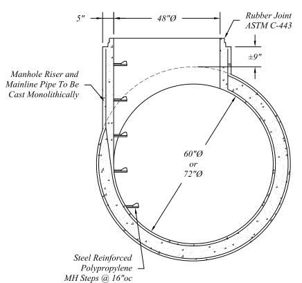
Pipe Manufactured To ASTM C-76 Specifications, Reinforcing Class As Required.
