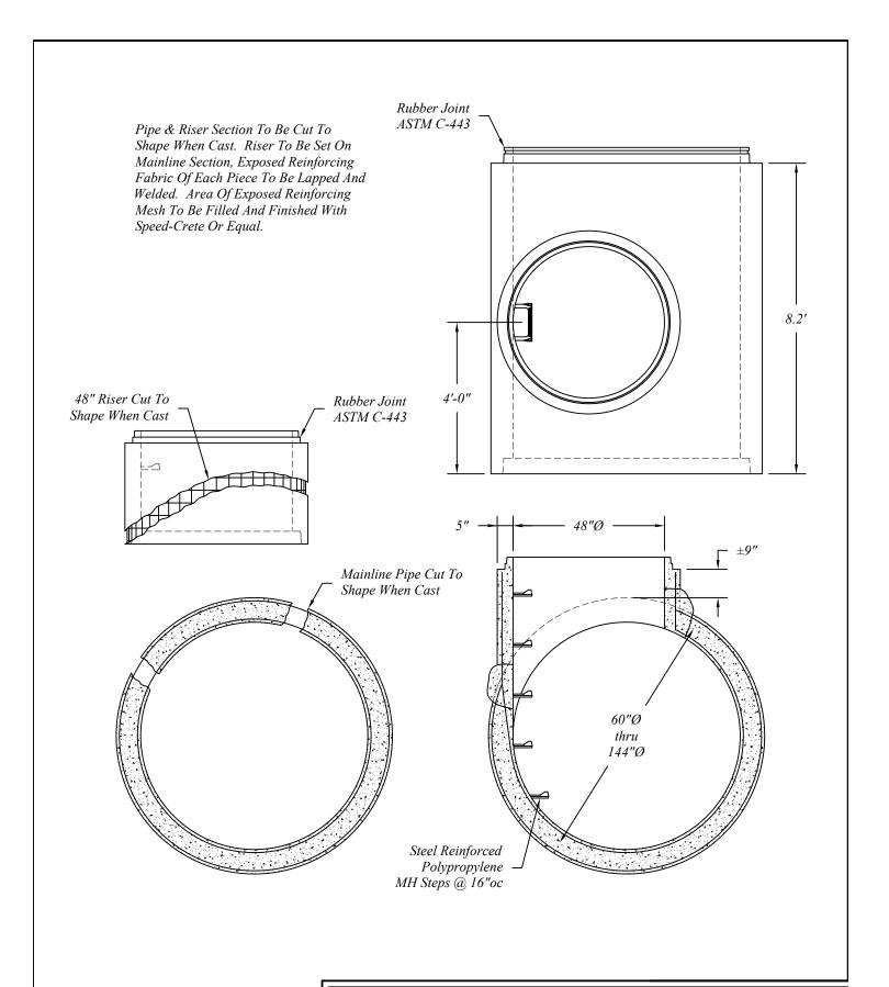
Pipe Manufactured To ASTM C-76 Specifications, Reinforcing Class As Required.
