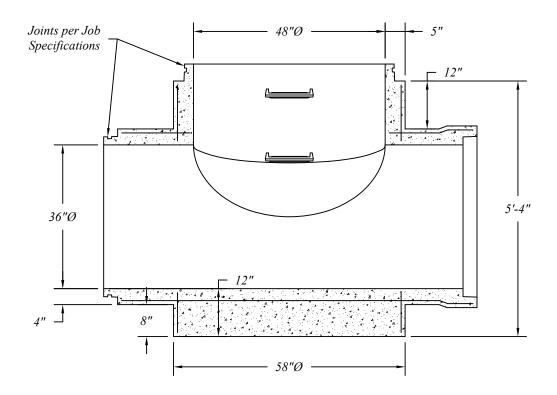
48" Riser Is Manufactured To ASTM C-478 Specifications.
