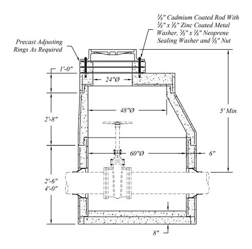
Gate Well Sections Manufactured To ASTM C-478 Specifications.
