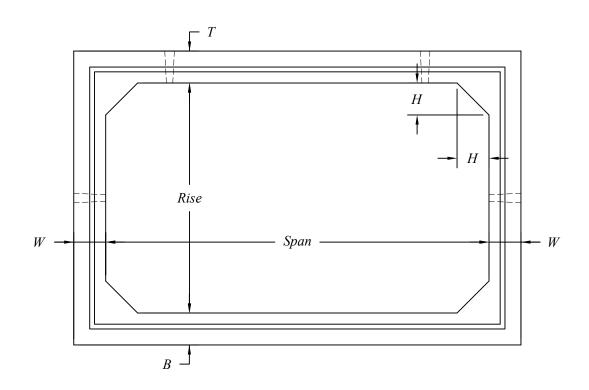
Box Culverts Sections Are Manufactured To 'ET Culvert' And/Or Applicable ASTM C-1577 Specifications According To Specific Project Requirements.
