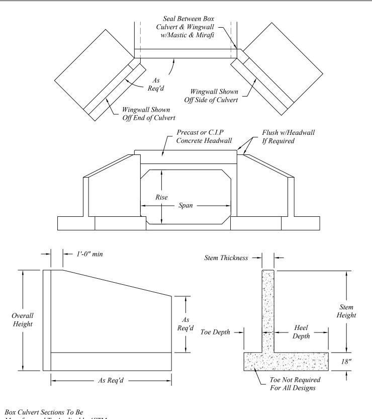
Box Culvert Sections To Be Manufactured To Applicable ASTM C-1577 Specifications.
