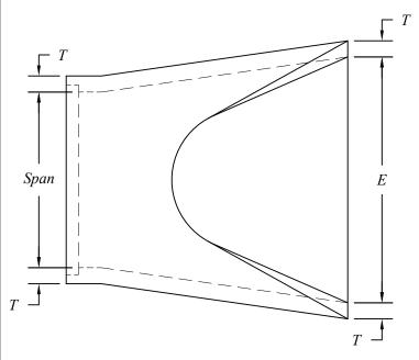
Precast Concrete Elliptical Flared End Sections To Be Manufactured To ASTM C-507-III and AASHTO M-207 Specifications.
