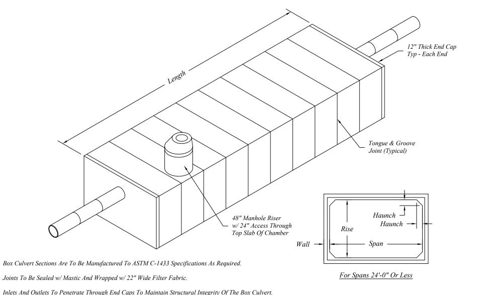
Inlets And Outlets To Penetrate Through End Caps To Maintain Structural Integrity Of The Box Culvert.
