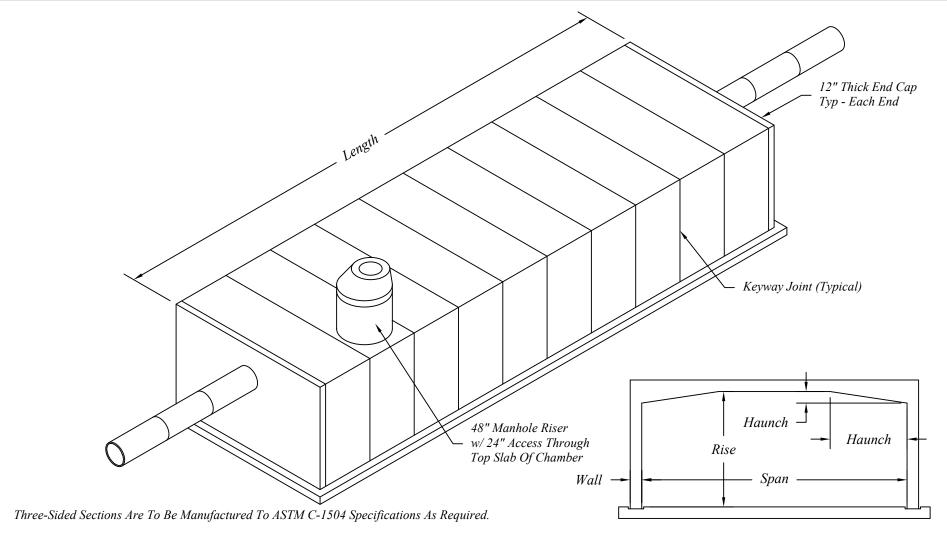
In Traffic Areas w/Less Than 2' of Cover, Non-Shrink Grout Must Be Placed In The Top Deck Keyway Only. Joints To Be Sealed w/EZ-Wrap or Equal and Covered w/22" Wide Filter Fabric.
