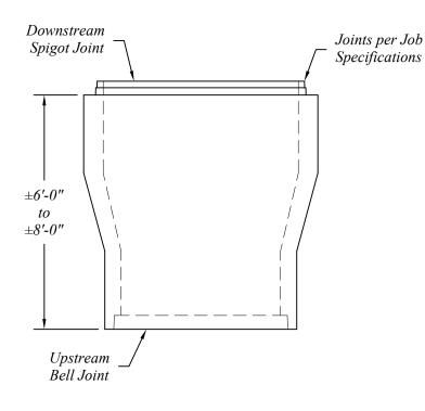
A 2' Section Of Each Required Size Of Pipe Will Be Poured w/6" (Min) Of Exposed Reinforcing Mesh. The Greater Of The Two Required Steel Areas Of Reinforcing Mesh Will Be Used In The Transition Portion Of The Segment. Additional #5 Bar @ 12" C-C Will Be Placed Length Wise On Both Reinforcement Cages For The Entire Length Of The Segment. All Reinforcement To Be Lapped And Welded. Exposed Area To Be Filled And Finished With Speed-Crete Or Equal.
