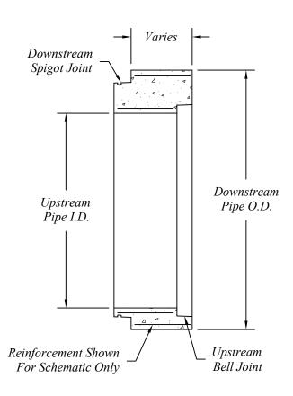
Flat Slab Transitions Are Manufactured To ASTM C-76 Specifications. The Reinforcing Used Shall Be The Greater Of The Two Required Steel Areas Of The Mainline Pipe.
